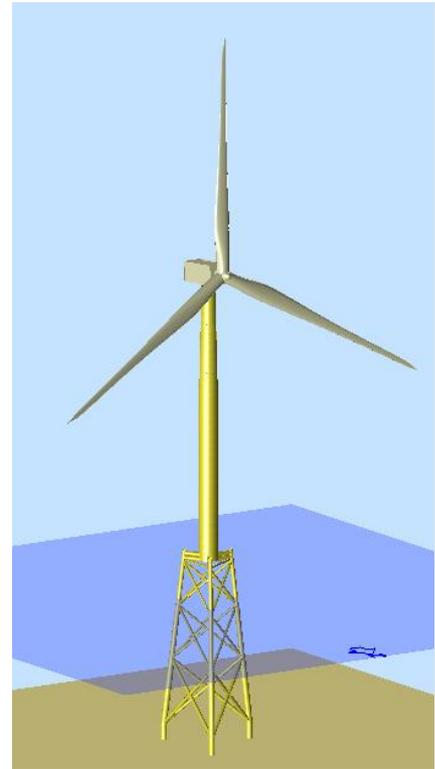
**Figure 5.1: Combined turbine and support structure model in Bladed.**
