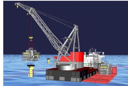
**Figure 6.4: Lifting operations in Sima.**
