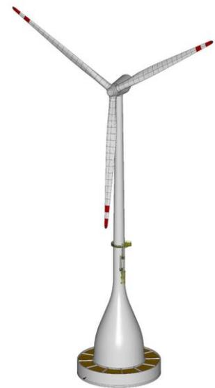
**Figure 4.8: Concrete GBS support structure.**
