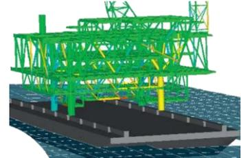
**Figure 6.2: A large topside on a barge.**
