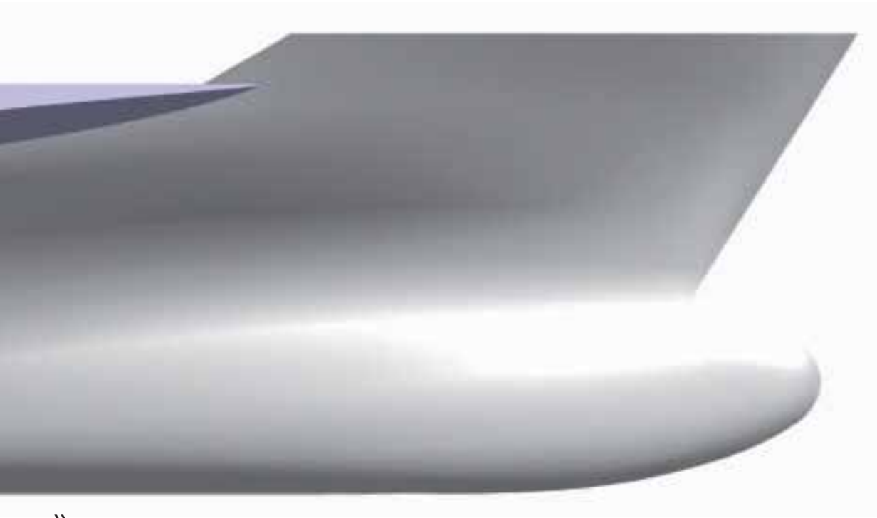
Fig.7: Final bow profile is slender and raked, to soften head seas.
