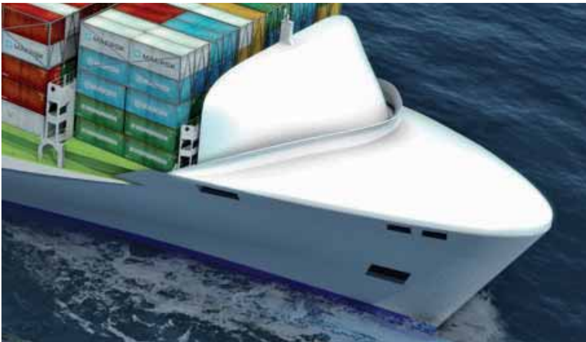
» Wind deflector and wave breaker build in GFRP.
