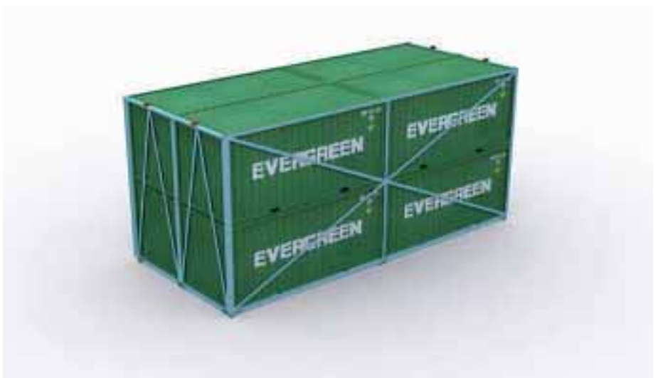
Fig.1: Frame structure for empty boxes capable of carrying eight 20-foot containers, four 40-foot containers or combinations thereof.
